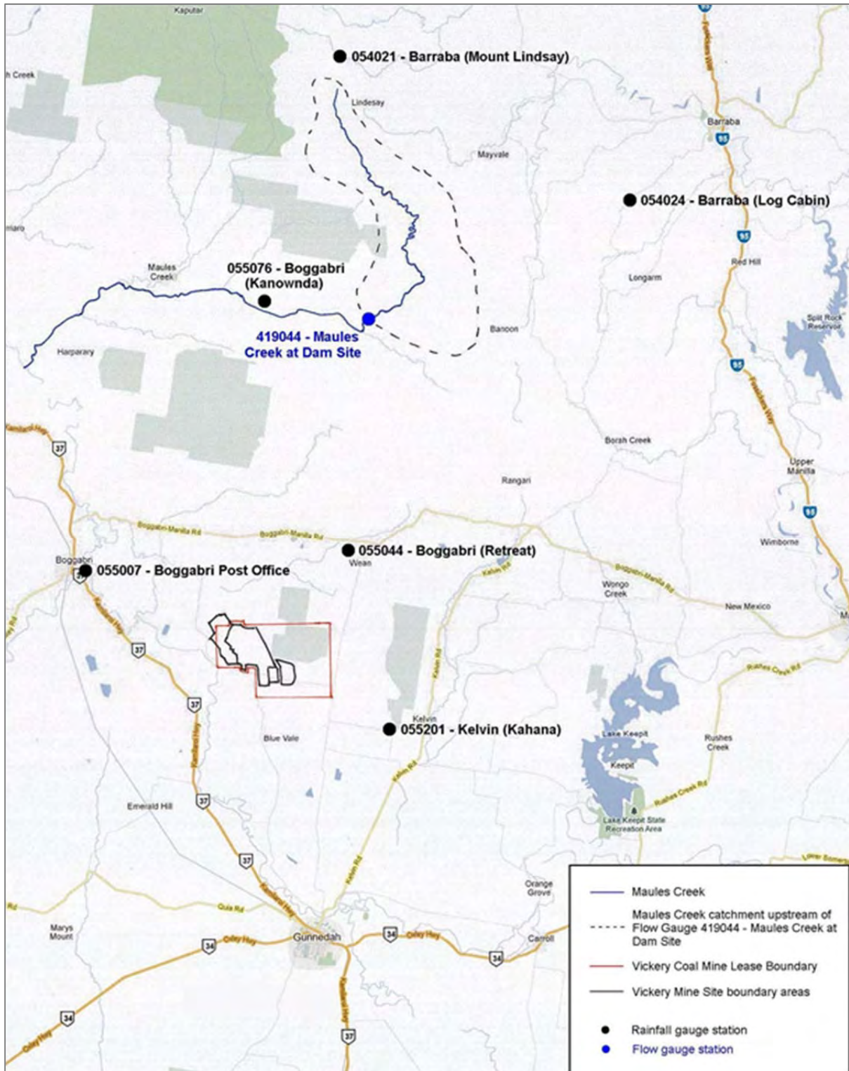
Figure 1: Location of rainfall and flow gauges used for calibration, validation & Project Area modelling
